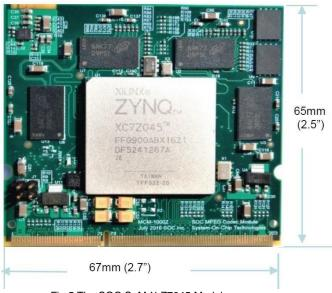
Fig.5 The SOC SoM-X-Z7045 Module
